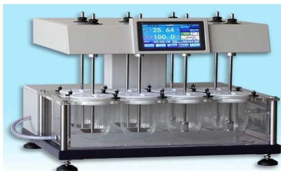
Figure 2.6. Drug Dissolution tester
