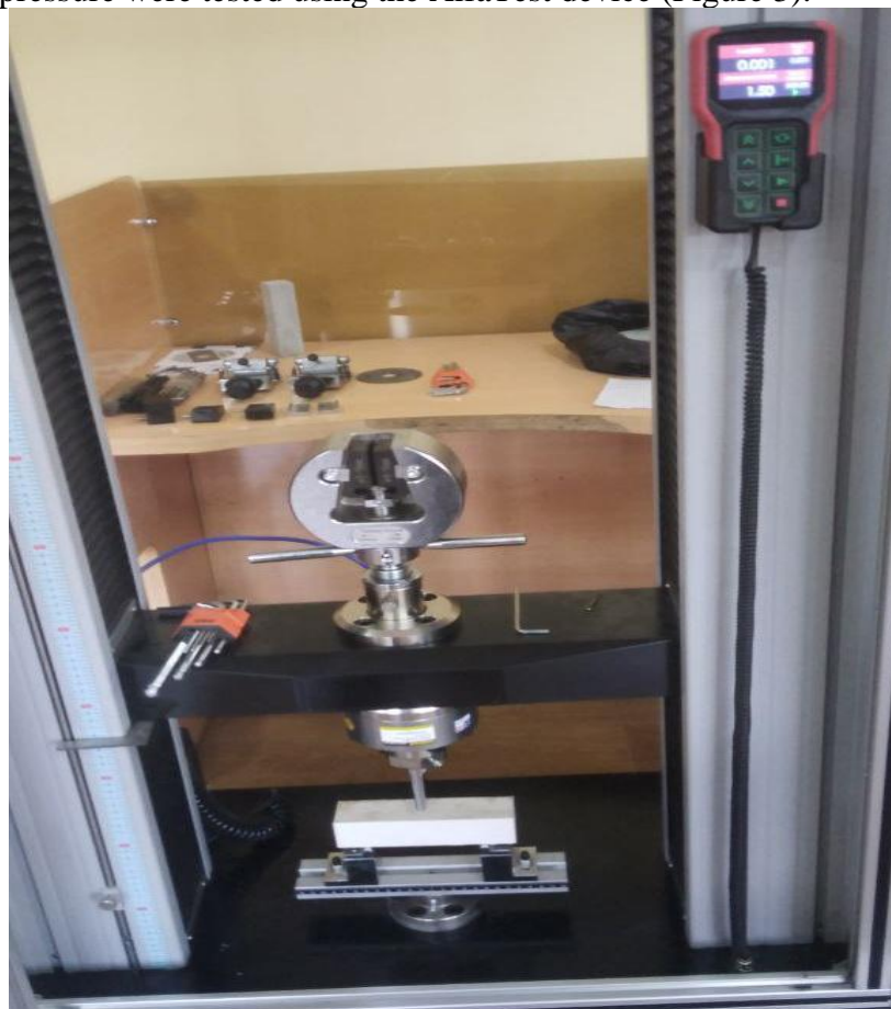
Figure 3: Testing for compressive and flexural strength using the AlfaTest device
