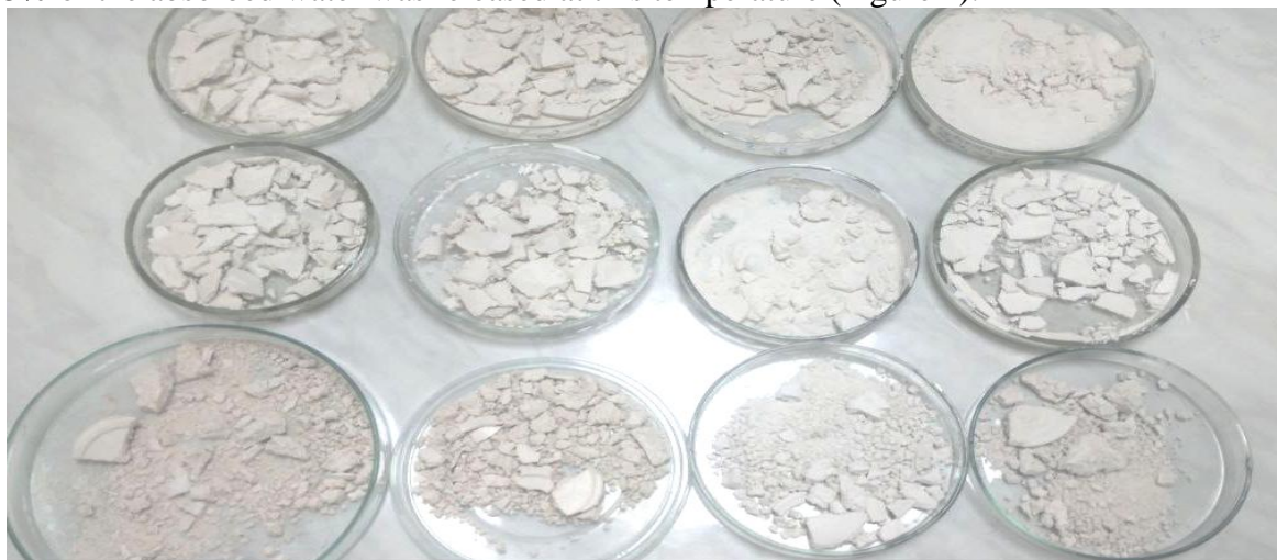
Figure 1: Samples taken at different temperatures to remove water from waste gypsum.
