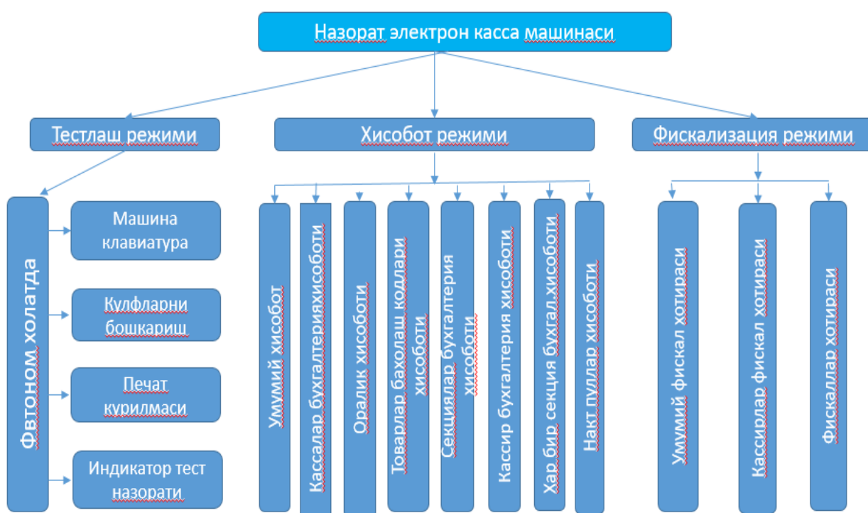
Figure -1. Operation of the control electronic cash register machine in different modes.
