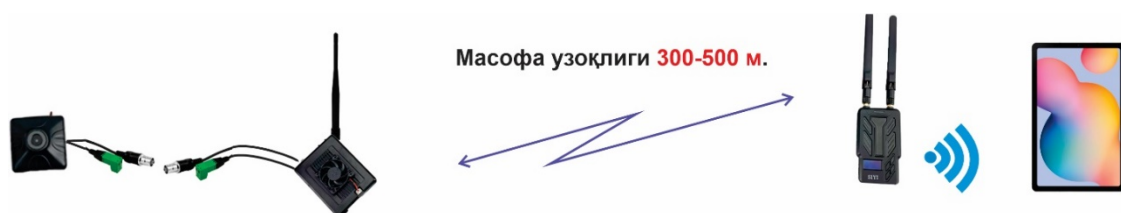
Figure 5. Video surveillance system connection diagram.
