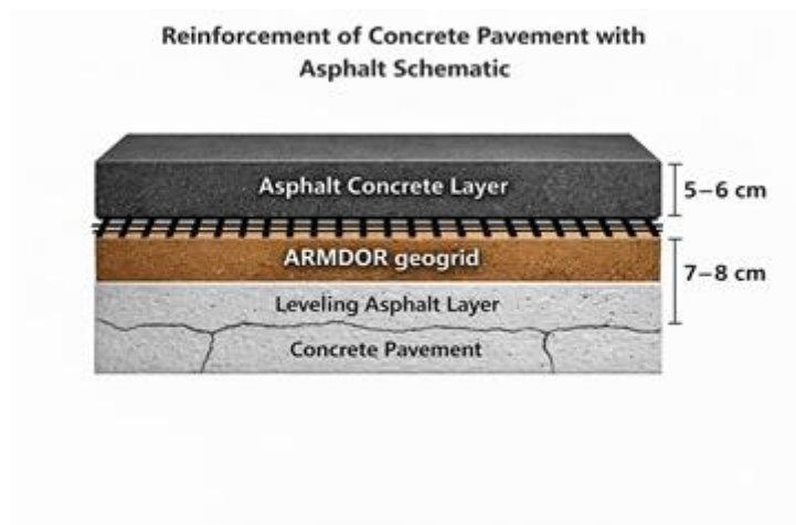
Figure 1. using the "Armdor" geogrid Reinforcement of cement concrete pavement with asphalt concrete using a leveling layer device: 1 - asphalt concrete reinforcement layer; 2 - expansion joint; 3 - "Armdor" Geoset; 4 - leveling layer; 5 - old cement concrete pavement; 6 - support; 7 - lower soil
