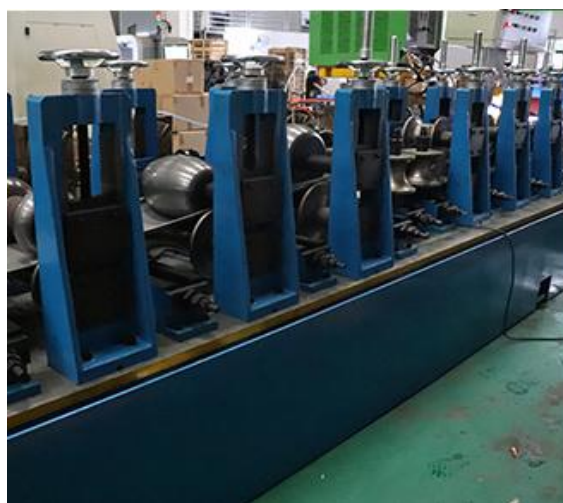
Fig. 4. Pipe forming mill: a - pipe forming stands; b – model of the pipe forming stand
