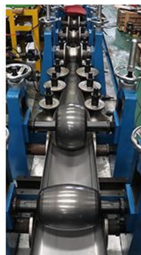
Fig. 4. Pipe forming mill: a - pipe forming stands; b – model of the pipe forming stand
