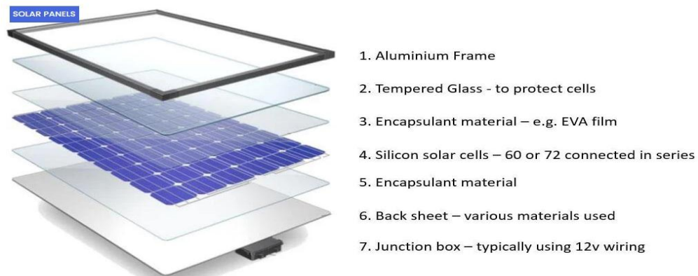
Picture 1. Structure of a solar panel.
