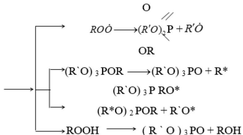
Organic phosphites of the aliphatic series interact with hydroperoxides at significantly higher rates than aromatic ones. Organic compounds containing sulfur interact with hydroperoxide
