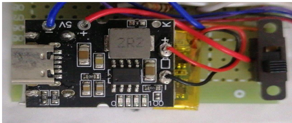
Figure (13) Connect the charger with the switch
