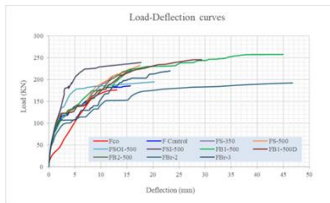
Figure 7: Load-deflection Curves for investigated frames
