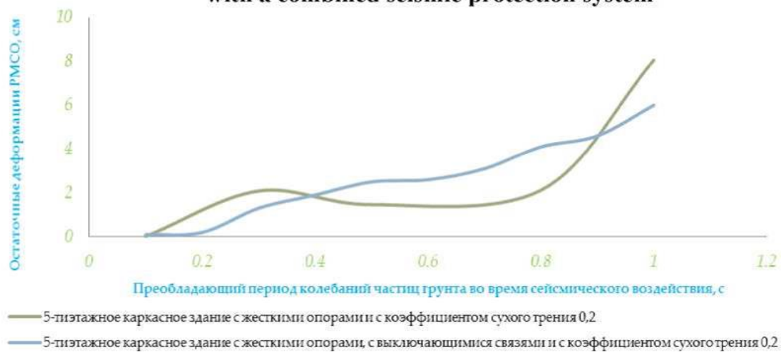
Fig. 7. Graphs of the dependence of the maximum residual displacements |y_0|_3 of the prevailing period of soil oscillation for 5-story frame buildings with a combined seismic protection system
