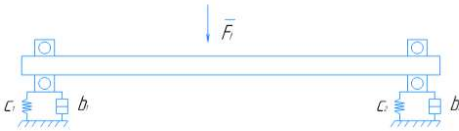
Figure 2. The scheme of the support of the propeller shaft with a belt bearing.
