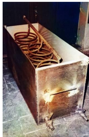
Fig. 2. General view of the installation for determining steam consumption
