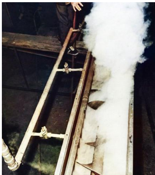
Fig.1. Steam supply to the mixer
