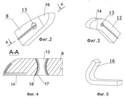
The recommended design of the looper of a sewing machine allows increasing the reliability of the loopers and ensures the production of high-quality stitches.
