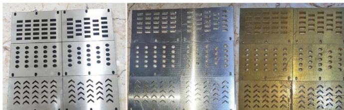
**Figure 12: Specimen designs materials and perforation shapes. [42]**
