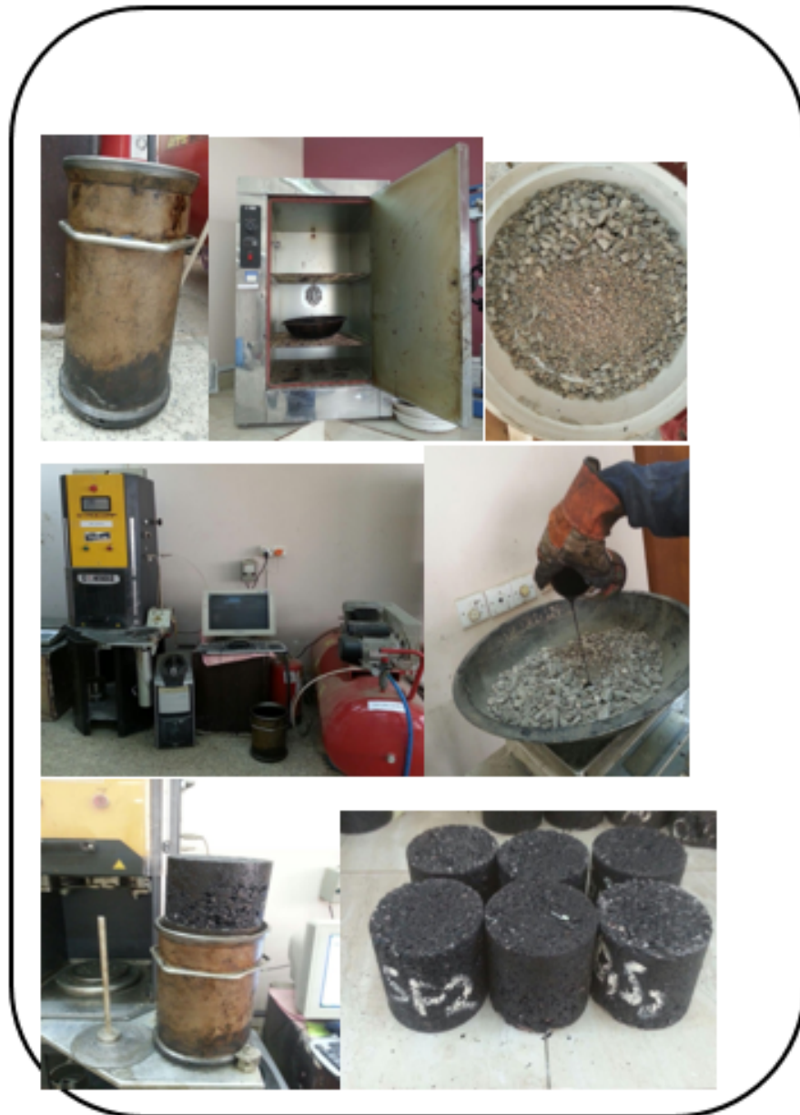
Plate (2): Preparation the specimens by use Gyrotory Compactor
