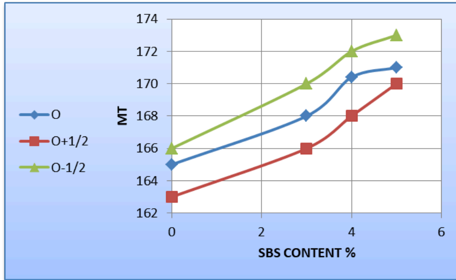
Figure (15): association between SBSC % and mixing temperatures for lime stone dust
