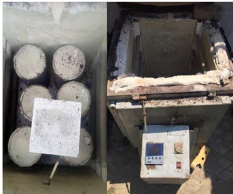
Figure 2: column CFST in the oven with samples of concrete cubes
