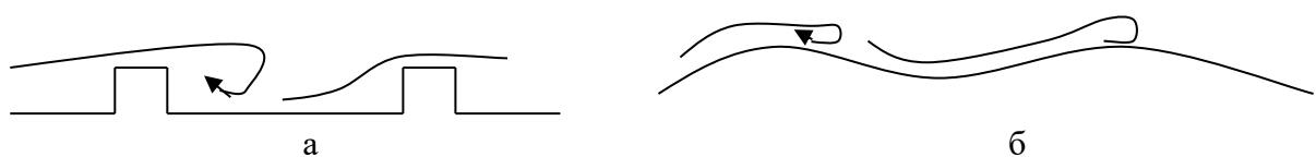
Fig. 1 Scheme of periodic renewal of the hydrodynamic boundary layer on the solar receiving surface: a – channel with roughness protrusions, b – wavy channel.
