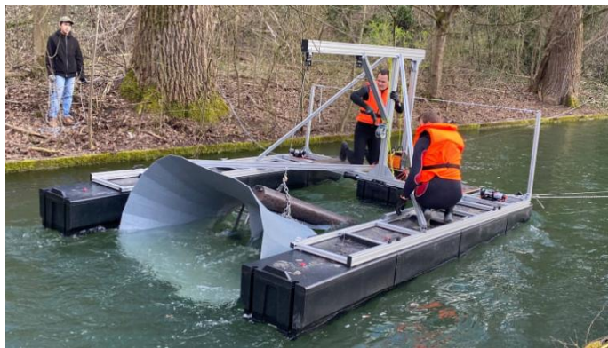
Fig.2. General view of a pico turbine on a pontoon base.
