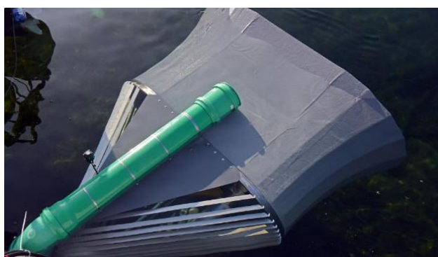
Fig.3. General view of a submersible hydraulic turbine with general guide nozzle [8]
