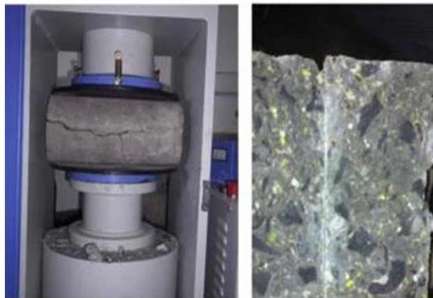
Fig. 3: Split tensile strength test of concrete
