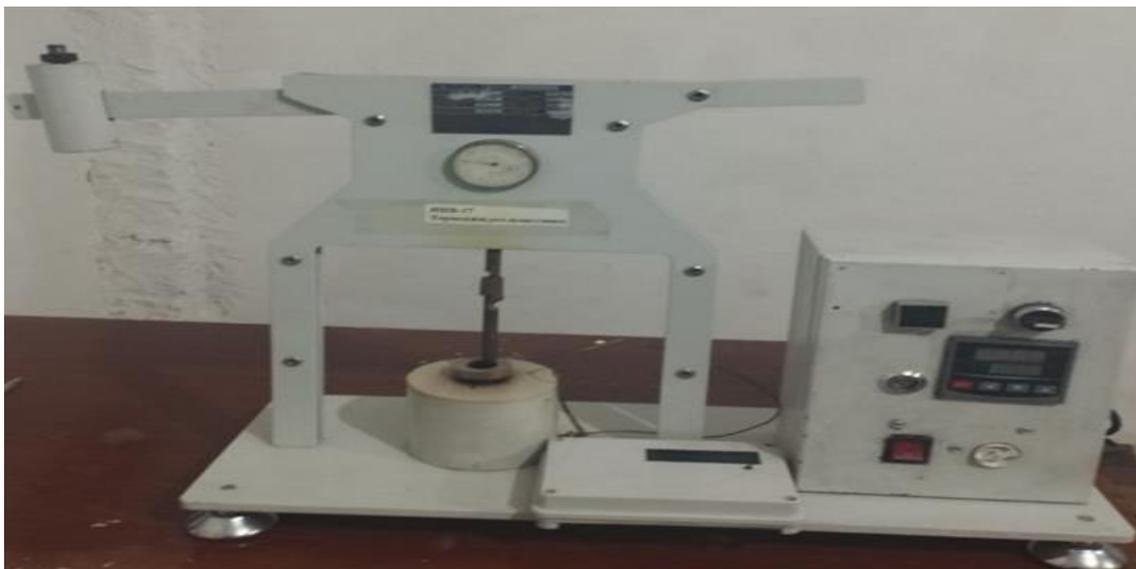
**Figure 2. Thermomechanical analyzer INV-17**
