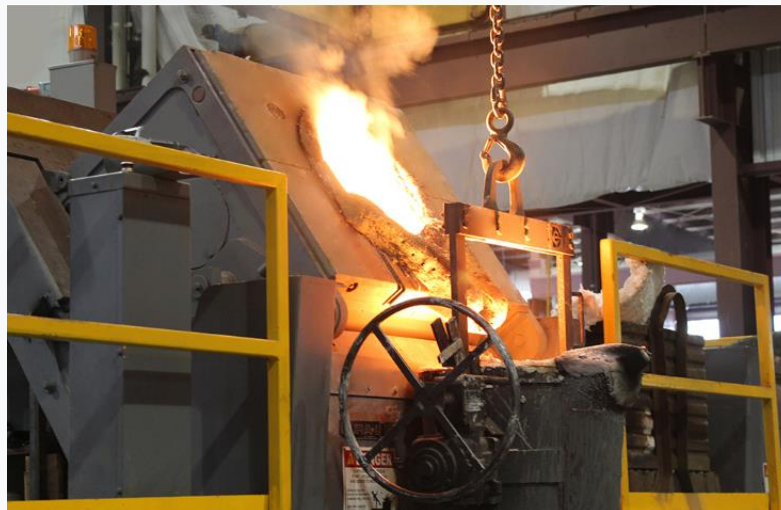
1 – picture. The process of ladle liquid metal from an induction furnace [35]
