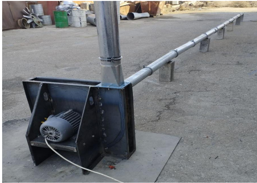
Figure 1. Experimental pneumatic transport equipment.
