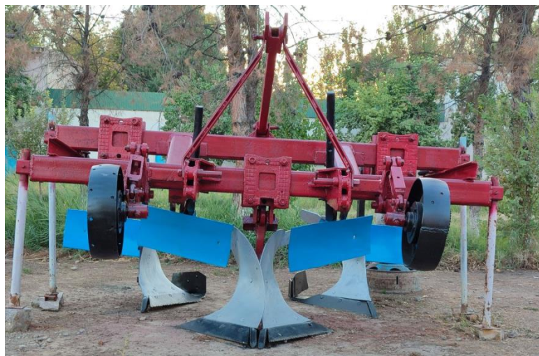
Figure 4. An experimental copy of a flat plow plow without an edge in closed and semi-open cutting conditions
