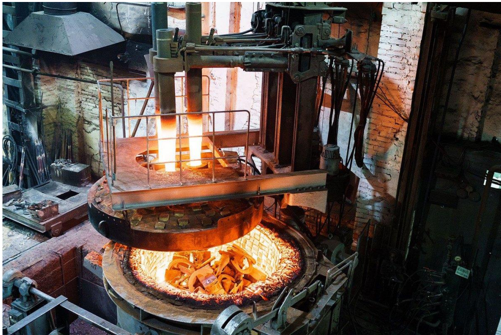
1 – picture. The process of loading solids into an electric arc furnace
