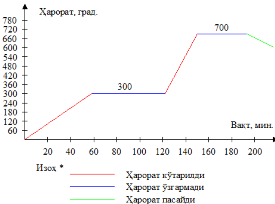
3 pictures. Graph of primary baking of hard alloy sample.
